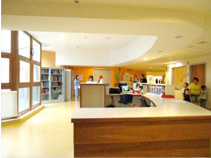
Figure 3.1: Nursing Station at Meyer Children's Hospital, Florence Italy. Natural light is brought in from two sides to this workstation; from one side, a small lightwell brings daylight deep within the building to a space that is essentially underground. From the other side, light comes in from a children's play-area, also providing a view outside.
